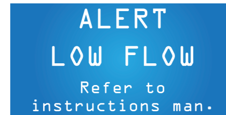
#5 PRIORITY Low Flow This message appears when the water flow is equal or below the factory-set minimum. For further instructions visit www.fluval-g.com .
