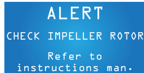
#2 PRIORITY Blocked Impeller This message appears when the impeller is blocked and the filter is not pumping water. For further instructions visit www.fluval-g.com .
